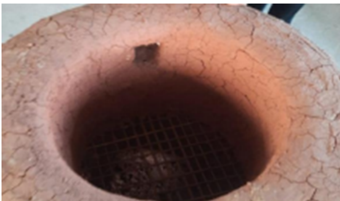
Figure 4: A furnace in which the mould is heated
